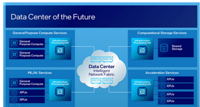
Figure 4: IPUs Support the Data Center of the Future
